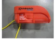
• Remove LED cap by removing 2 off Screws.
