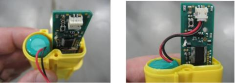
• De-press the battery counter reset button, the LED and buzzer will operate for a duration of 1 second when indicating a successfully reset.
