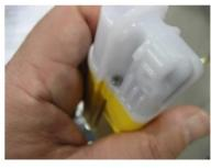
• Remove the battery. The PCB & foil insert do not need to be removed.
