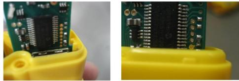
• Fit battery assembly into casing, care should be taken to ensure foil insert is not damaged. Position the wires as shown. Connect the battery to the PCB.
