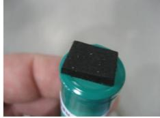
• Ensure the replacement Sealing Gasket is fitted to the replacement LED cap assembly. **Note**: Ensure the gasket is seated correctly or product may fail the leak test.
