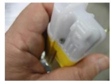
• Perform an ON/OFF test by pushing and releasing the 'On' button. The beacon should flash at least once and a beep should be heard with each flash. Switch off the beacon by pushing and holding the 'Off' button – the
