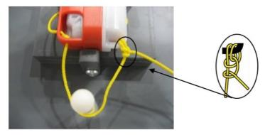
Rigged for semi-automatic operating according to the lifejacket manufactures guidance notes. When preparing the unit ready for lifejacket semi-automatic activation it is not necessary to tie of the lanyard to the white section as this will be done by the lifejacket installer. The free end of the longer length of the lanyard need not be attached at this time.
