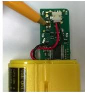
• Fit LED cap - ensuring the wires are not trapped; secure with 2 off Screws. Tighten to 60cNm.
