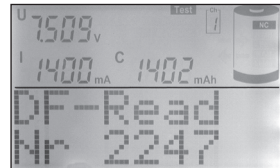
Fig. 34: Reading out the flash data memory
