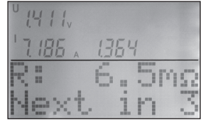
Fig. 23: Main Ri measurement function window
