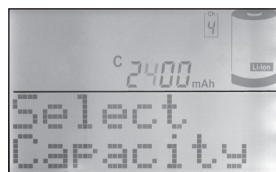
Fig. 13: Entering the nominal battery capacity
