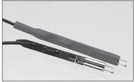
Fig. 1: Special measuring cables with spring-loaded probes
