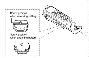
**NOTE:** When removing or attaching the battery pack, use a coin or standard screwdriver to loosen or tighten the bottom screw.
