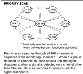
Set the TAG channels (scanned channels) before scanning. Clear the TAG for unwanted channels which inconveniently stop scanning, such as those for digital communications. (p. 15)
