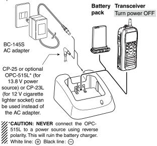
515L to a power source using reverse polarity. This will ruin the battery charger.
