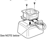
**NOTE:** Some of the PCB type desktop // charger adapters (incl. AD-75/88) do not need connection of the 3-pin connector. The connection is required only for the installing adapter that is compatible with charging a Li-Ion battery pack.
